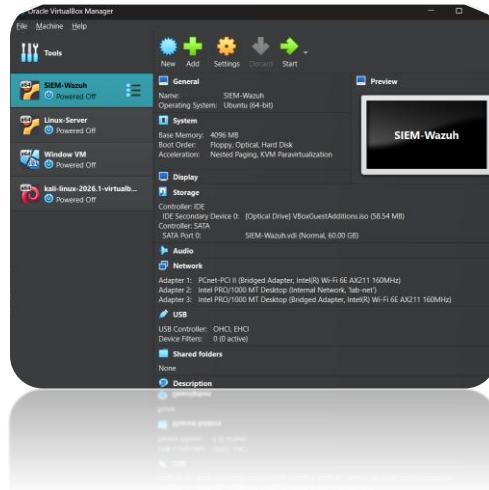
Figure 3. Wazuh SIEM virtual machine configuration and resource allocation.
